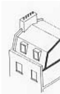
Early mansard roofs comprise a steep pitched roof, normally 70 degrees or greater, with a shallower secondary pitch above. In the first half of the eighteenth century these slopes were clad in clay tiles. Later, when slates were used, slopes could be lower and with the use of lead, the top of the roof could be almost flat.
