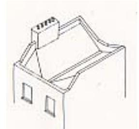
Butterfly roofs were usually concealed on the front façade of the building, by a parapet which blocked the two half gables and the gutter. On the rear façade, 'butterfly' roofs were often left visible, with the wall following the 'V' shape of the roof forming an interesting pattern crowning the back of the terrace.
